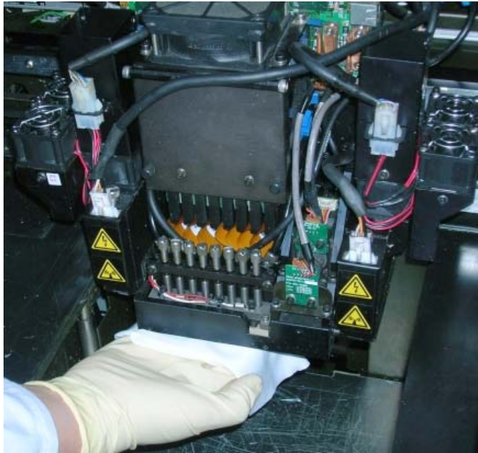
Figure 6-25: Cleaning the heads
